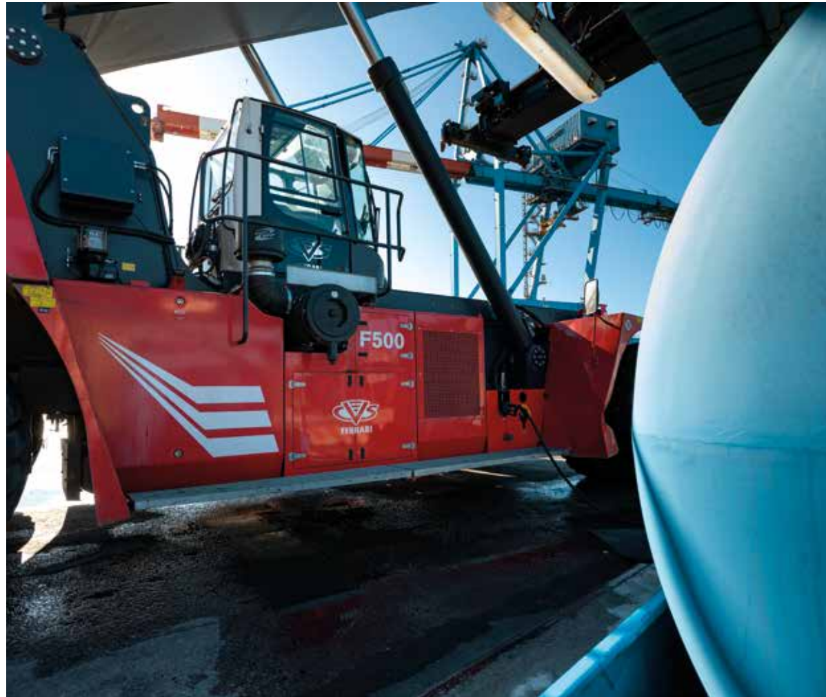
PSA SECH: urea filling station, an additive used to reduce nitrogen dioxide (NO x ) emissions.
