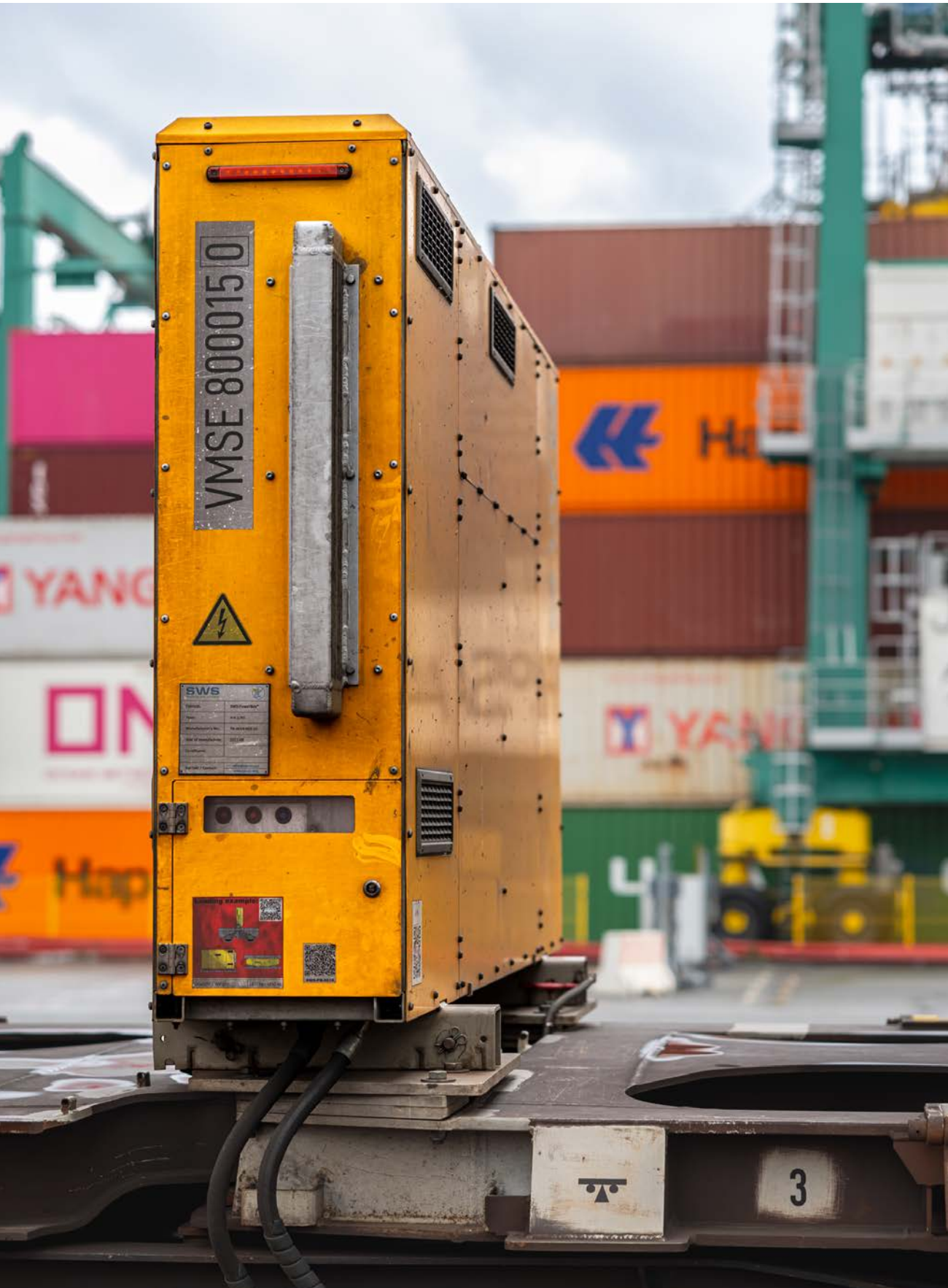
Reefer containers can now be shipped on the Southern Express train thanks to this power box
